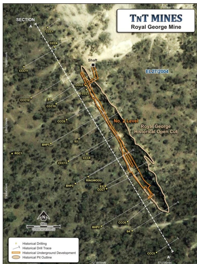
Figure 2 Royal George Open Cut and Drilling Plan
